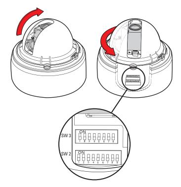
Figure 12. Locating the Spectra Mini Dome DIP Switches
